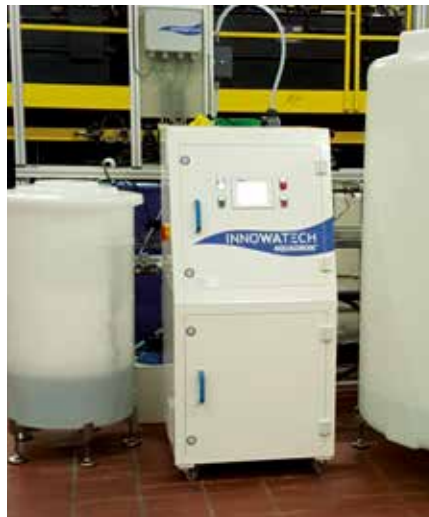
Left: Aquadron® PGK with salt-tablet reservoir (small container) and Anolyte supply tank (large container) for coolant treatment. pH-neutral Anolyte is being produced in INNOWATECH's electrolysis cells (on the right).
