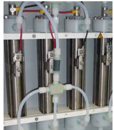
Left: Aquadron® PGK with salt-tablet reservoir (small container) and Anolyte supply tank (large container) for coolant treatment. pH-neutral Anolyte is being produced in INNOWATECH's electrolysis cells (on the right).
