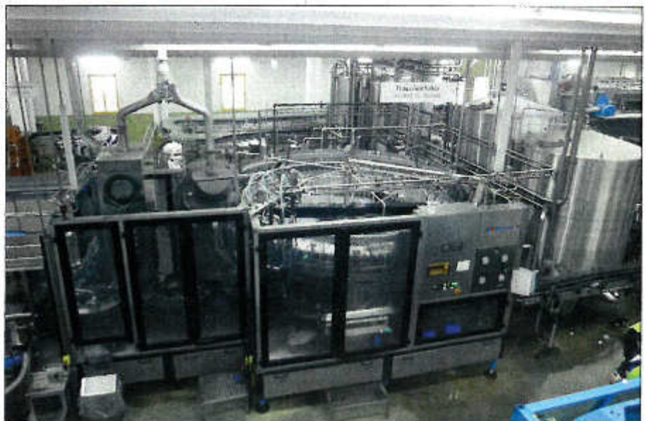
CIP disinfecting of the mixer (left) and filler (right) constituted the second step in the changeover to the Innowatech Anolyte disinfectant.
