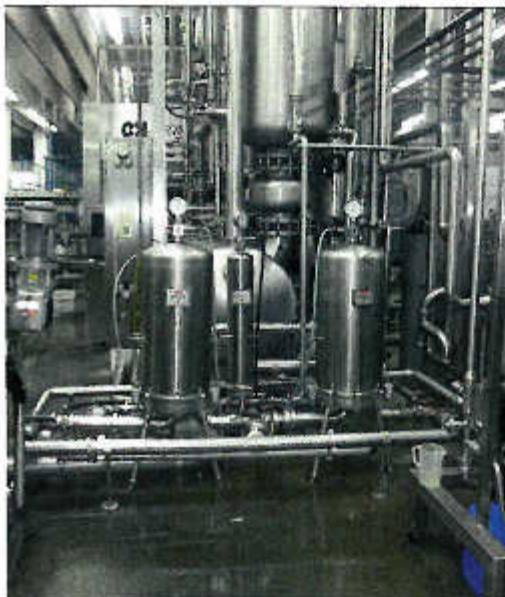
CIP disinfecting of the mixer (left) and filler (right) constituted the second step in the changeover to the Innowatech Anolyte disinfectant.
